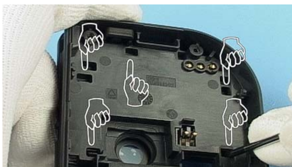
Lock out the snaps of the IHF lid carefully.
