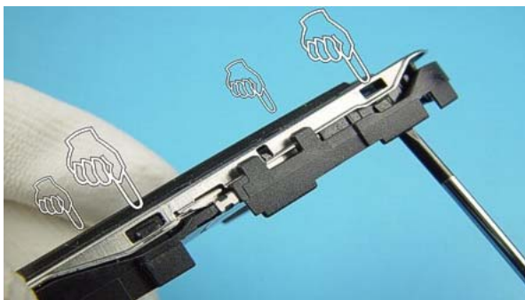
Use a slotted screwdriver to unlock the snaps of the LCD top shield assy on both sides.
