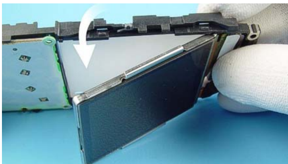
The LCD module drops out when turning the UI-frame.
