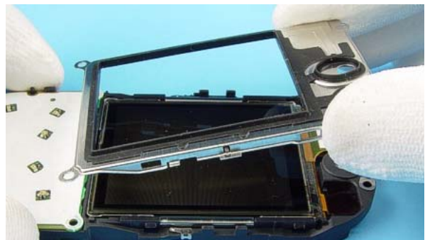
Now, the LCD top shield assy can be removed.
