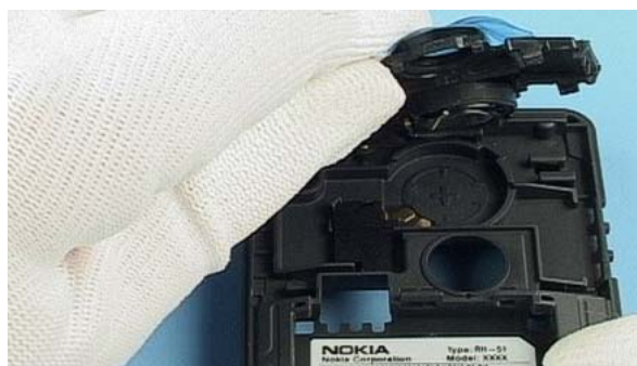
Turn the B-cover as shown in the picture and remove the IHF lid.
