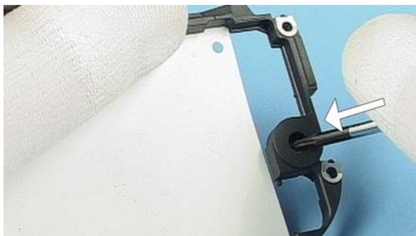
The earpiece can be removed from its guidance by pushing with TORX screwdriver through the B-cover.
